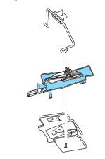
If you are stowing the flat tire, remove the L-shaped bolt from the external pocket of the felt bag. With the 3rd row seat in the raised position, stand the flat tire in the rear of the vehicle with the tire's valve stem facing the rear of the vehicle. Fasten the flat tire to the vehicle by inserting the L-shaped bolt through one of the lug bolt holes in the wheel and turning
